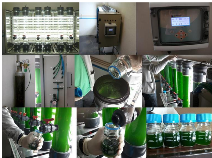
1 2 3 FIGURE 3 Culture in column PBR installed in the University of Aveiro and 4 extraction of samples 5
