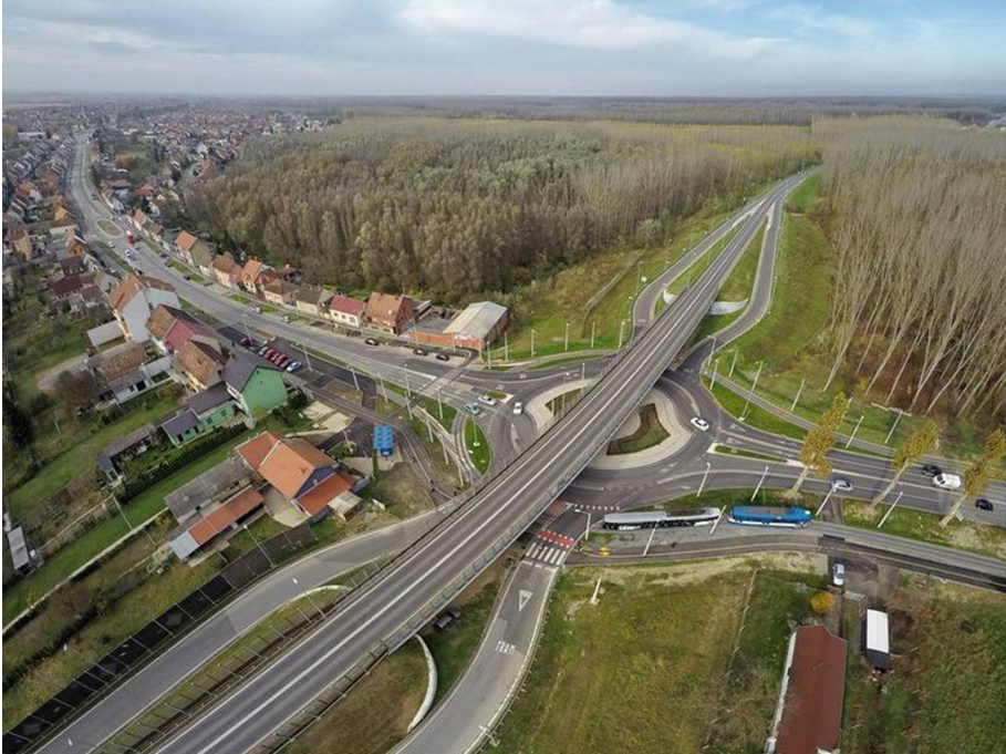
Fig. 3. Turbo roundabout in the City of Osijek, Croatia - in traffic 2014
